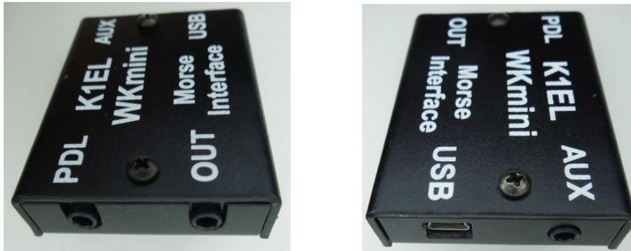
There are four connectors on WKmini, two on the left side and two on the right, The left facing connectors are labeled PDL and OUT. The PDL connector is an 1/8" stereo jack which accepts paddleset input. The paddle can be an iambic or side swiper type. A bug is not acceptable. The paddle inputs are activated when switched to common ground (GND). The paddle connector needs to be wired this way:
